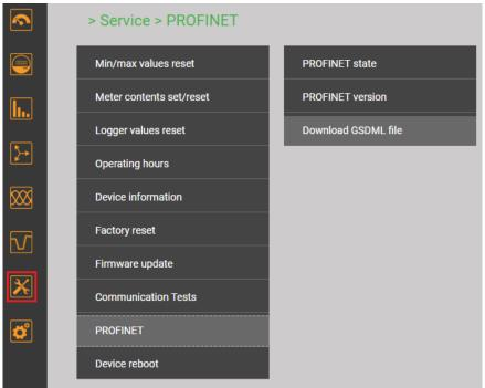
Before a device can be used in a project, the associated GSD file must be imported in the configuration tool (e.g. TIA Portal).
