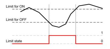
Using limit values either the exceeding of a given value (upper limit) or the fall below a given value (lower limit) is monitored.
