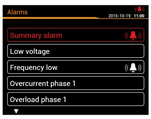
The digital or relay output assigned to the summary alarm can be reset by means of the <OK> key. So the active alarming will be stopped. But the alarm state of the summary alarm remains active until the alarm state no longer exists.
