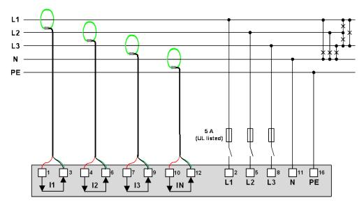
When connecting the coils you must follow the safety notices given in the operating instructions of the Rogowski coil. The current direction shown on the coils must match the real current direction and has to be the same for all phases.
