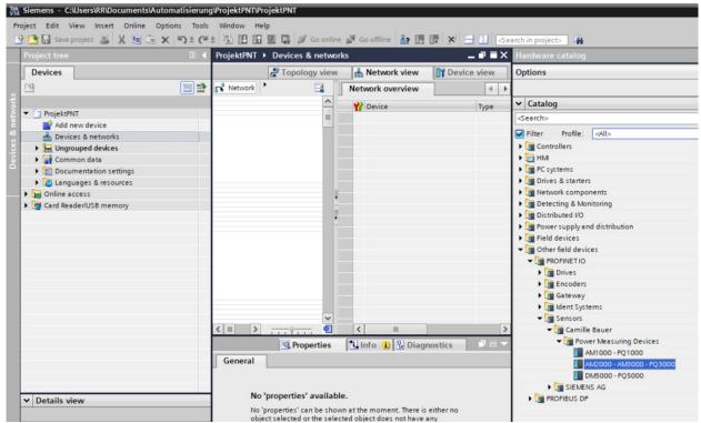
As soon as the GSD file has been imported, the device is available in the hardware catalog and can be integrated using drag&drop. There are three models available that represent the different designs of the whole device series. The selection shown above is for example suited for the devices AM2000, AM300 and PQ3000, which have the same design (panel 144x144mm) and support the same measured values.
