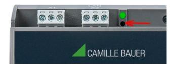
If the communication settings of the Standard interface are no longer known, they can be reset to the default settings by pressing the sunk-in reset button (located below the operating LED) for at least 3s. During the reset the operating LED flashes red. After the reset the device is rebooted.
