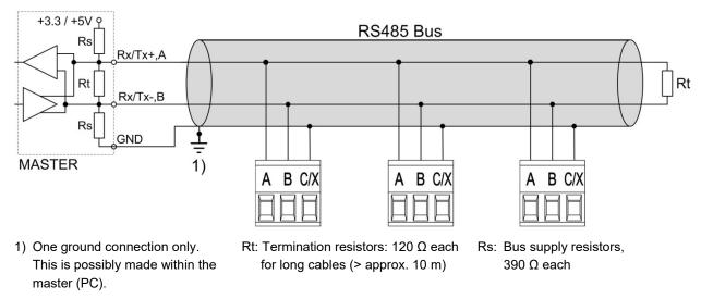
The signal wires (A, B) have to be twisted. GND (C/X) can be connected via a wire or via the cable shield. In disturbed environments shielded cables must be used. Supply resistors (Rs) have to be present in bus master (PC) interface. Stubs should be avoided when connecting the devices. A pure line network is ideal.
