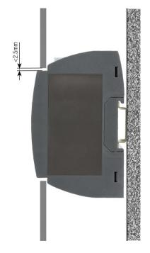
The device can also be mounted that the front of the device protrudes through a cut-out in the enclosure. So the operating buttons and the display become accessible. With centric mounting using the below maximum cut-out a gap between enclosure and device results, which does not exceed 2.5mm on each side.
